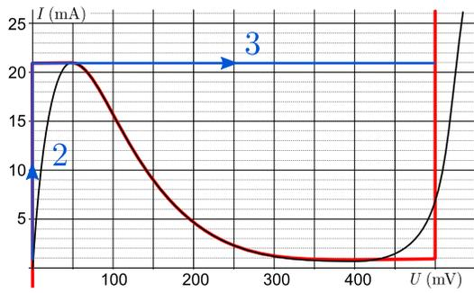
In leg 2 of the journey, the current increases from  $I_i = 0$  to  $I_i = I_2 = 21 \text{ mA}$  (measured from the figure). The time taken is  $t_2 = LI_2/\mathcal{E} = 4.2 \times 10^{-8} \text{ s}$ . Since in leg 3, the change in current is 0, the time taken is essentially instantaneous compared to  $t_2$ . Hence  $t_3 = 0$  for our considerations. The total time taken is then
